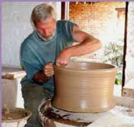
Pulling up the walls
