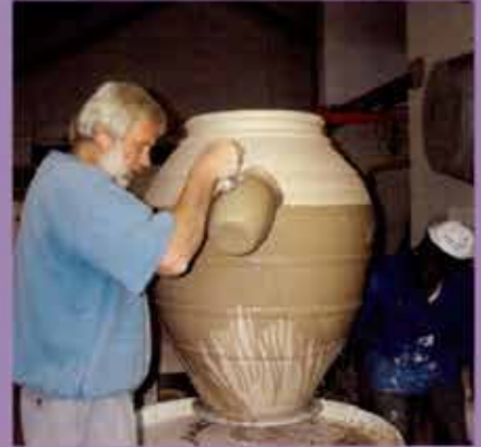
Pouring the glaze, starting at the base
