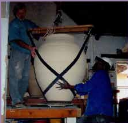
Pot is lifted in harness to kiln using a hoist
