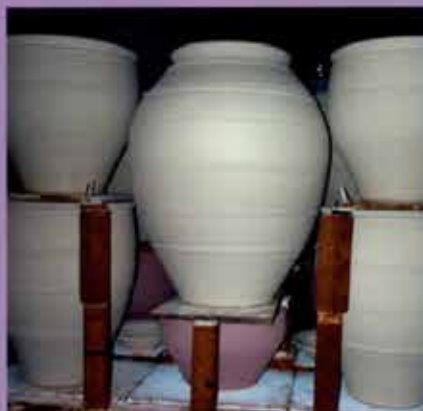
Fully loaded trolley kiln ready for firing
