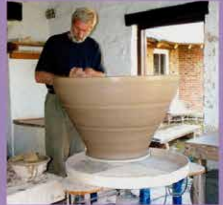
Finishing the rim of the third section
