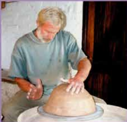
Securing clay on wheel
