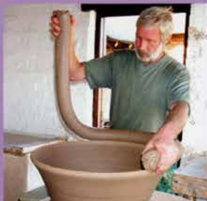
Laying the coil on the rim
