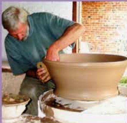
Ribbing the walls outwards
