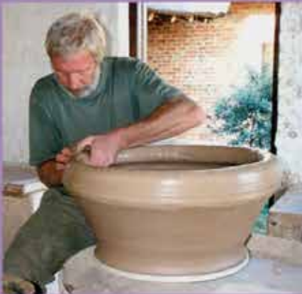
Controlling the coil
