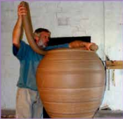
DAY SEVEN: Adding final coil for the rim
